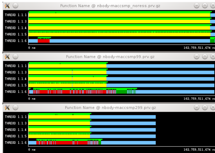
Figure 3: Comparison of the executions of Nbody with and without the resources extension on Jetson
