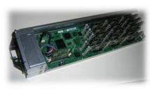
Each Mont-Blanc compute card integrates one Samsung Exynos 5 Dual SoC, 4 GB of DDR3-1600 DRAM, a microSD slot for local storage and a 1 GbE NIC, all in an 85x56mm card (3.3x2.2 inches). A single Mont-Blanc blade integrates fifteen Mont-Blanc compute cards and a 1 GbE crossbar switch, which is connected to the rest of the system via two 10 GbE
